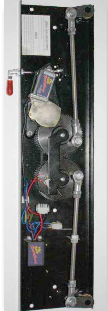
HEADER MECHANISM USED FOR 360 ENTRANCE DOORS
